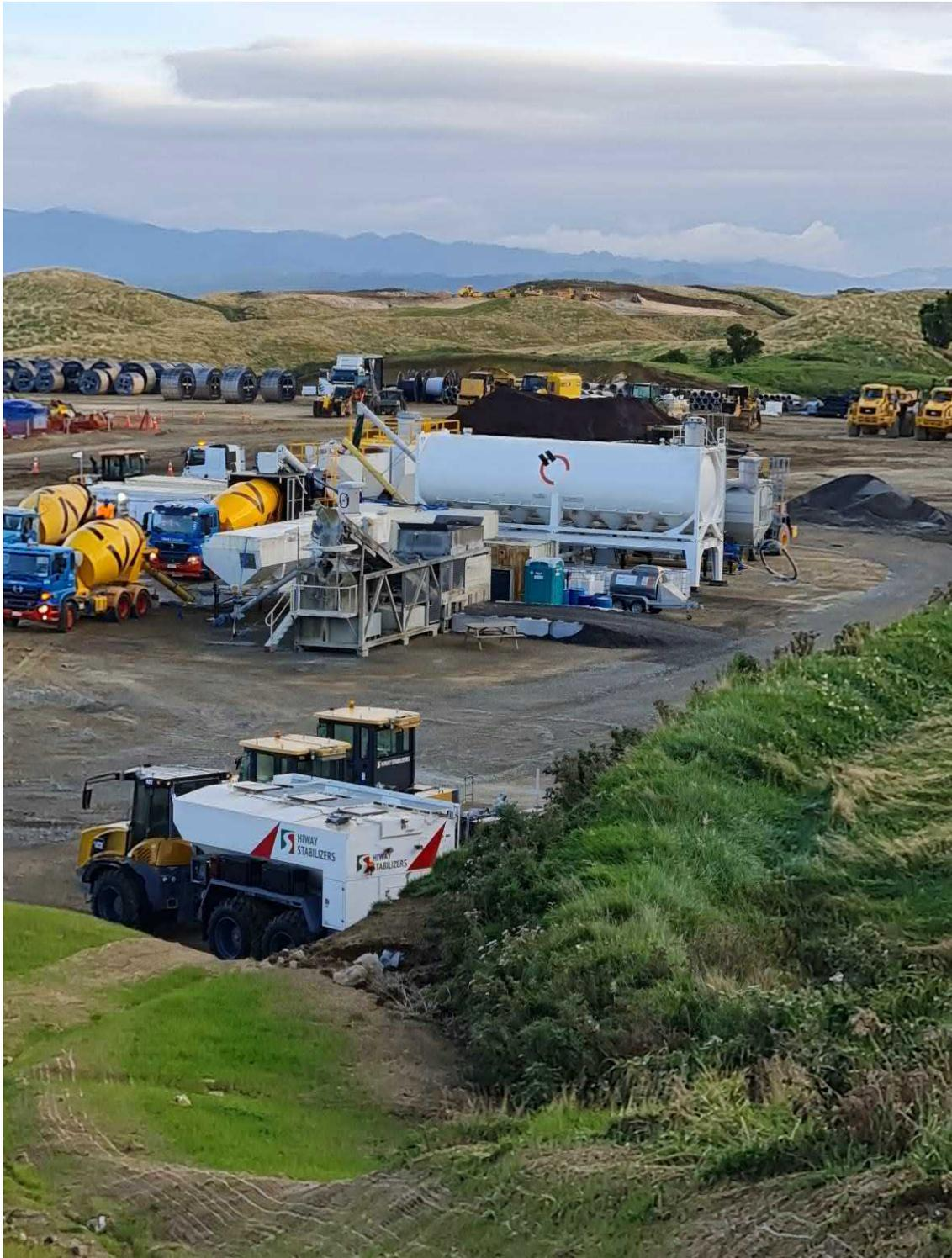
**Figure 3: Concrete Batching Plant**
